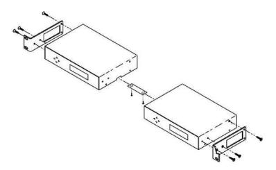
When mounting two components in one RU rack space, use the two short rack ears and the tie bar assembly. Note that the QDA4-45 and QCA9-33 have solid side panels and should not be mounted next to components with the ventilation holes, as that will block airflow.
